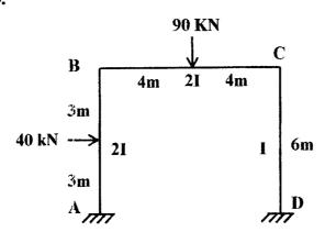
Q.6 (a) Analyse the beam shown in figure by stiffness-method.
